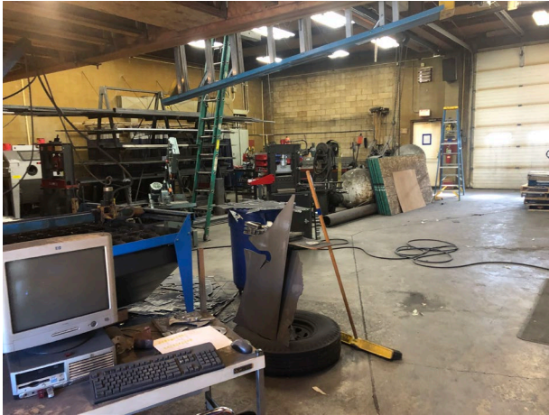
Metals shop lacks equipment Exposed CMU exterior wall little or no Insulation.
